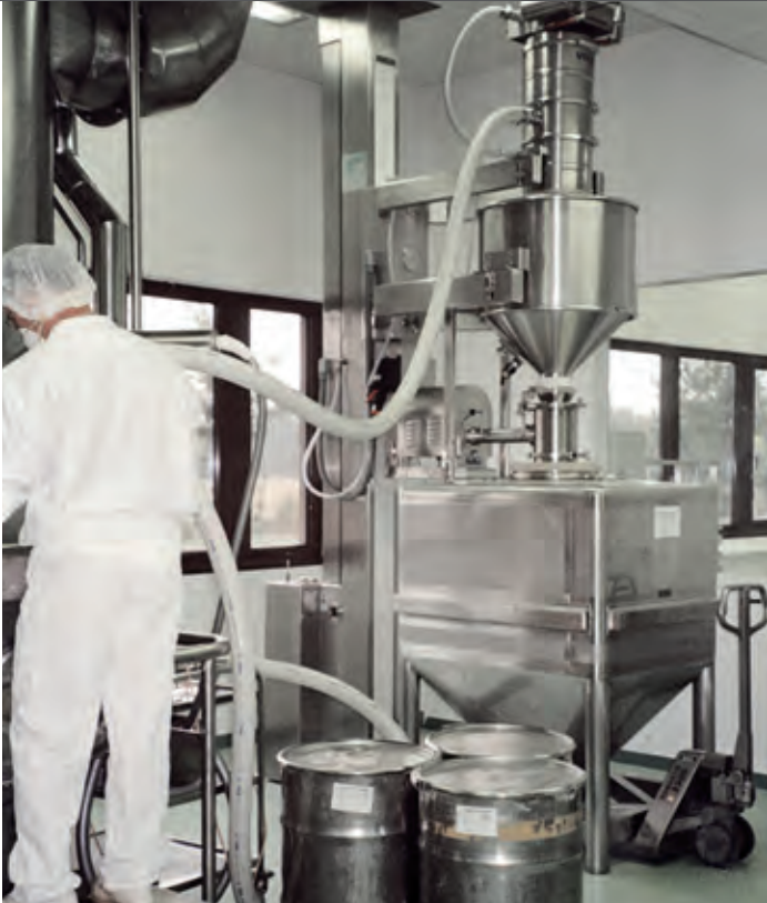
Emptying a dryer with a manual suction wand.
