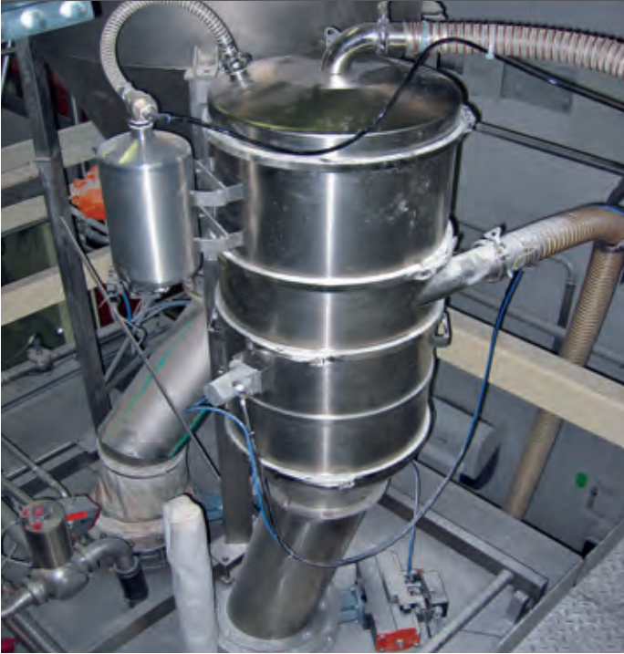
Vacuum conveyor in the food industry for conveying additives.
