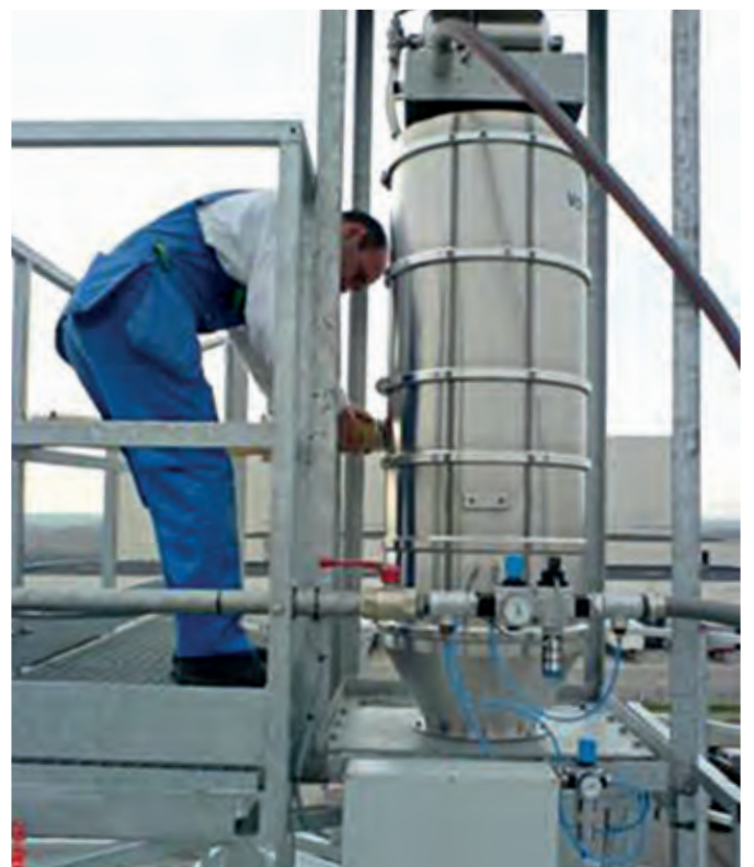
Vacuum conveyors in an outdoor installation, for charging silos.
