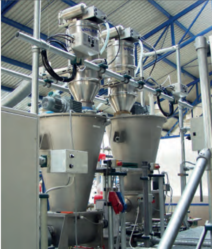
Two vacuum conveyors for loading loss-in-weight feeders.
