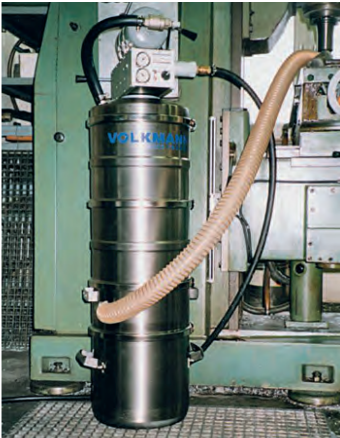
Industrial vacuum cleaner for picking up swarf
