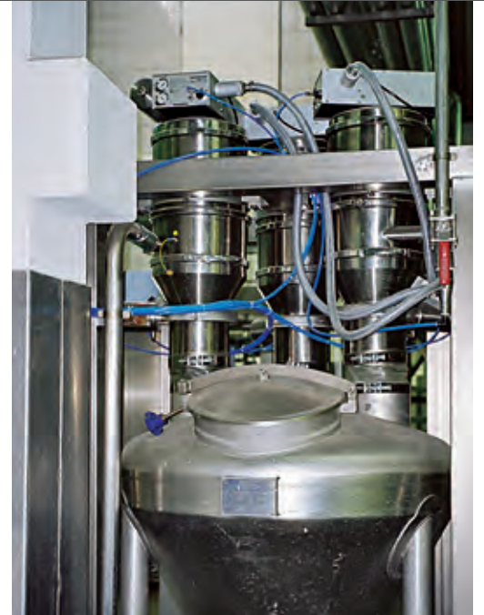
Conveying of cake/bread mixtures in the food industry.
