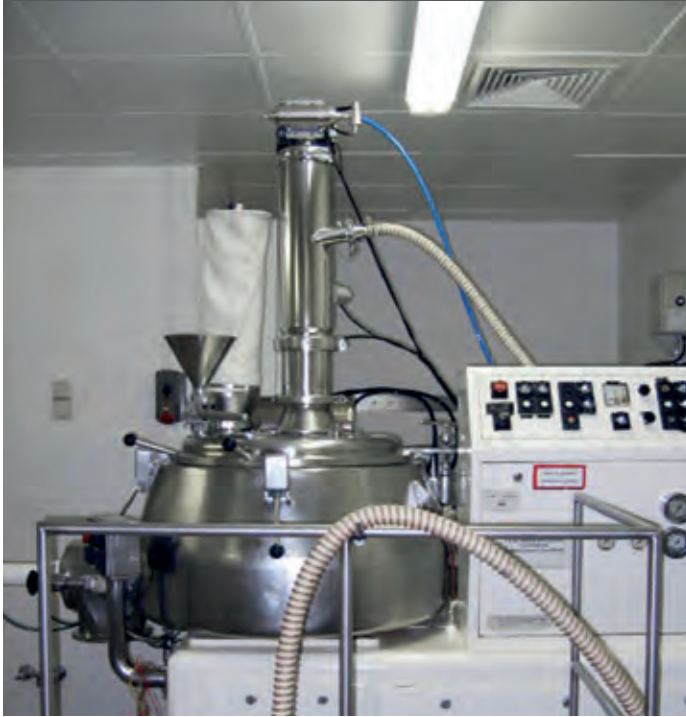
Loading of the mixer using PPC.
