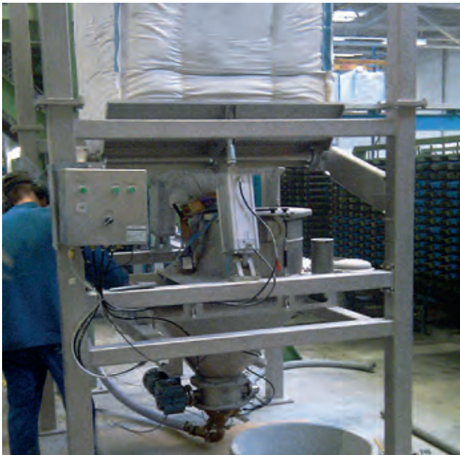
The bulk bag emptying station in the construction industry with massagers and lump breaker for products which do not flow easily.
