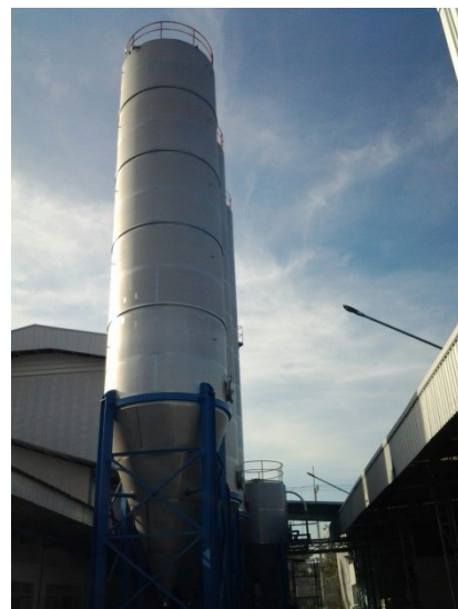
Silos Weighting system (PVC powder & Calcium Carbonate Powder ) Saha Area , Twin Lion brand PVC pipe factory
